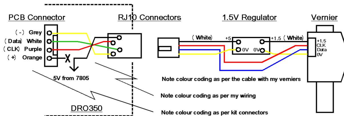
Apologies for the mixed colour codes which confuses. As drawn the wiring follows through as seen with top view of the PCB connector, bottom view of the RJ10 socket, mating orientation of the RJ10 plug and top view of the PCB regulator and the Vernier scale.
