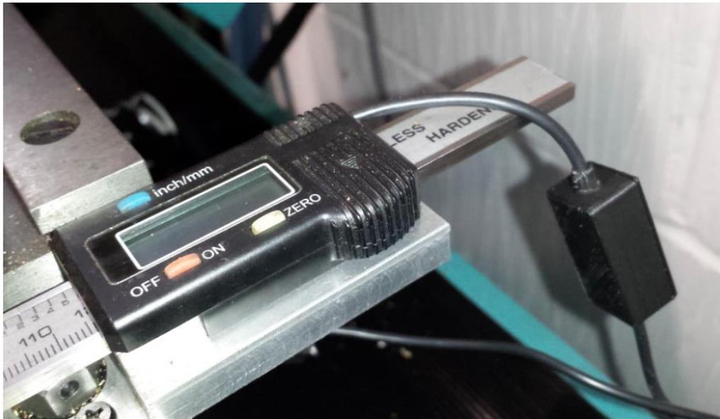
So far so good. I now had a 1.5V regulator connected close to the scale connections which if I ran from a 5V external power supply gave me stable readings on the DRO350.
